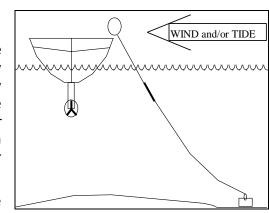
Fix the length of the line so there is little or no excess line floating around.
